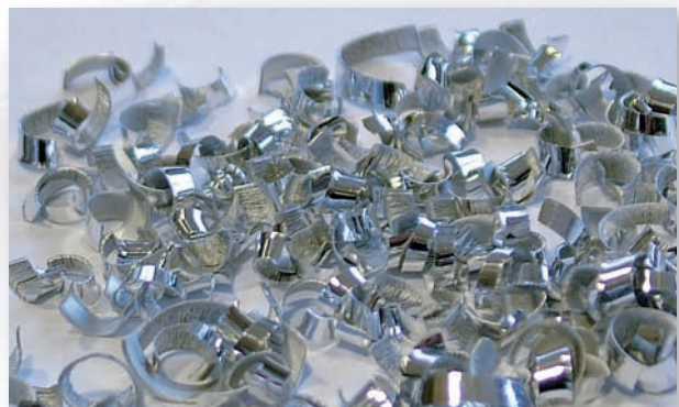
With 3D-chip breaker: Breakage chips
