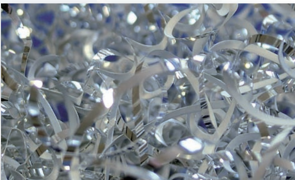
Without 3D-chip breaker: Flow chips
