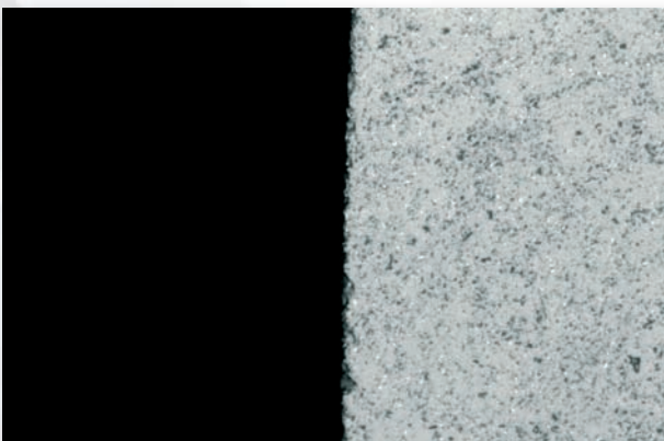
Magnification 500 x: PDC-Finest grain size, ground super fine
